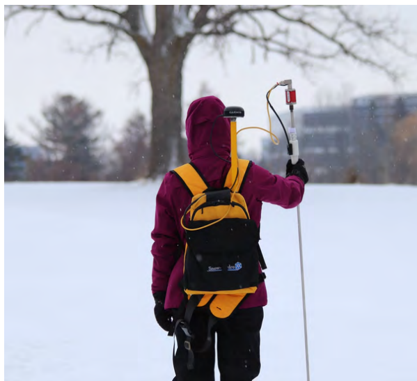
During the workshop, students had the opportunity to gain hands-on experience using modern tools for measuring snow and ice. Shanlin Boychuk used the Magnaprobe (pictured here) to conduct a snow survey transect. Photo credit: Branden Walker
